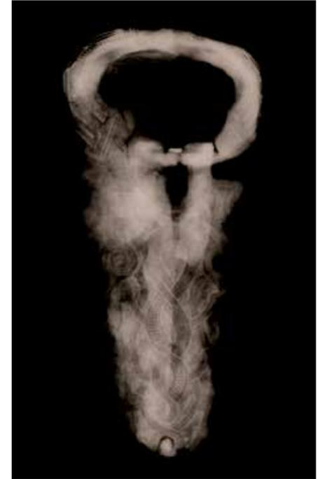
**X-ray examination** is a method that uses the ability of X-rays to penetrate materials. Different materials absorb X-rays to different extents. For this reason, the shape of metallic objects as well as certain manufacturing and decorating techniques made of noble metals can also be made visible under the corrosion layer.
